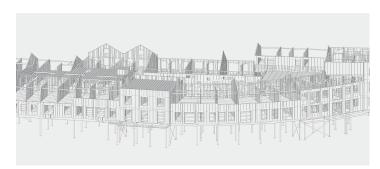
Sigmat helped the main contractor McCarthy & Stone to design and build a new superstructure to house retired over 60's in a stunning location which overlooks Weymouth Marina. We installed a hot rolled steel podium to form under-croft parking as well as communal areas. This dovetailed perfectly with the 3-storey Sigmat light gauge steel frame and the Sigmat Mansard roof.
