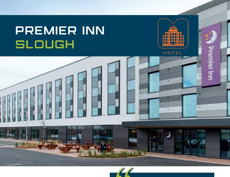
Sigmat were appointed by Bowmer & Kirkland to deliver the light gauge steel framing for the new Premier Inn in Slough. The scheme comprised of 5,690m2 of Sigmat panels, 4.9 tonnes of hot rolled steel members, 18 flights of stairs and 9 half landings.
